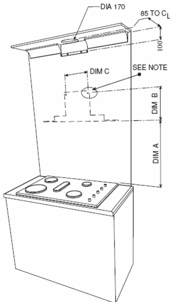
1. Pre drill pilot hole 3mm diameter at dimensions C and B. B=300mm and C=220
