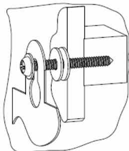
**NOTE:** Fixing to a solid stud is recommended.
