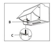
2. Whilst the front panel is still open, remove the two screws **(B)** and then press the tab **(C)** down and remove the front panel from its quide rails.
