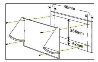
8. Place the front panel against the furniture door. Using the screws provided, secure the front panel of the rangehood to the inner surface of the furniture door.
