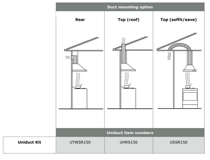
It is recommended that Ø150mm ducting is to be used, however a reducer from Ø150mm to Ø125mm is included with the rangehood should Ø125mm ducting be required.
