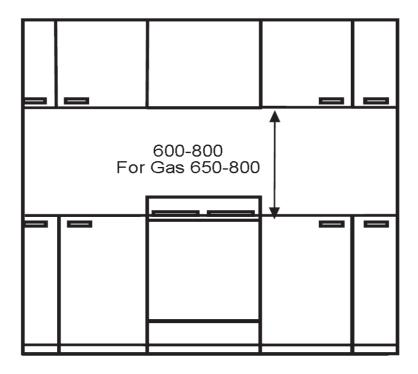
Pictured: Minimum height from the hob surface to the underside face of the rangehood is: 600mm for electric hob, 650mm for gas hob
