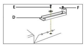
3. Secure the extractor mounting brackets **(D)** onto the top of the hood, using the screws and washers **(E)** supplied. Check that the adjustment screw **(F)** is fitted.
