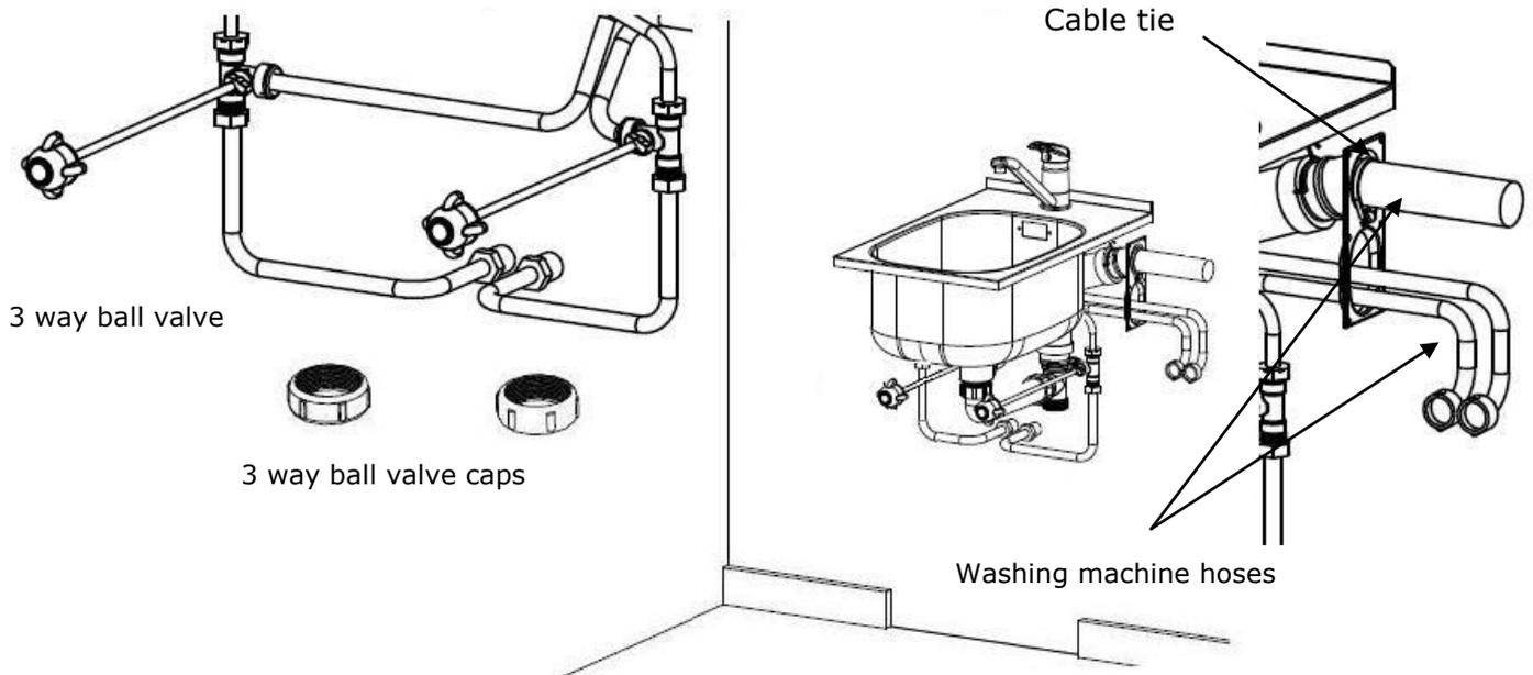
Confirm if the washing machine waste inlet needs to be moved from right to left before securing the unit to the wall. If they do need to be changed see page 6 of these installation instructions.
