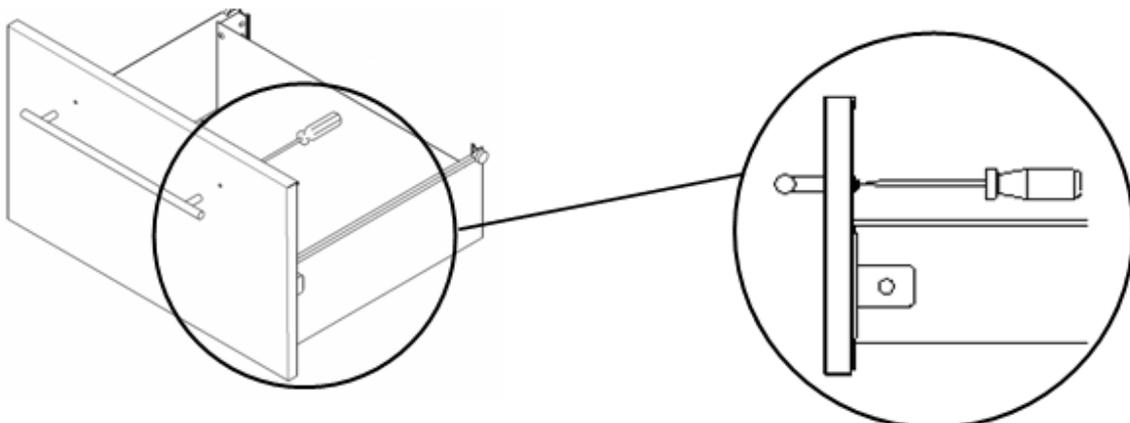
**3.** To fix handle to the drawer, firstly clear the existing holes from the front using the screws supplied. Insert screw & washer from the inside (back of the draw front) of the drawer, place handle on the outside of the drawer front and secure in two locations. Be careful not to scratch the drawer fronts whilst installing the handles.
