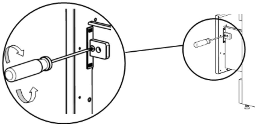
**2.** The handles are to be connected to all two drawers of the Robinhood laundry tub.
